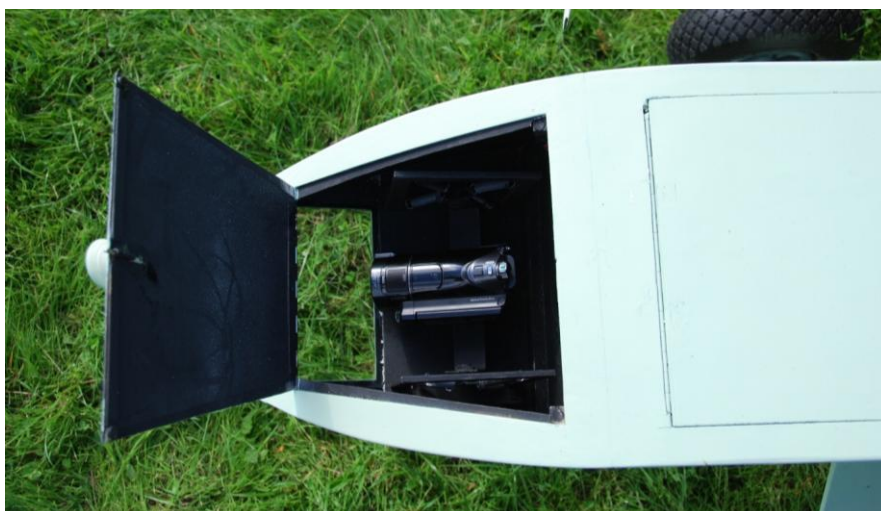
A high definition SONY camcorder is used on long range photographic reconnaissance missions to record the mission and augment the coverage of the digital cameras in the payload bay.
