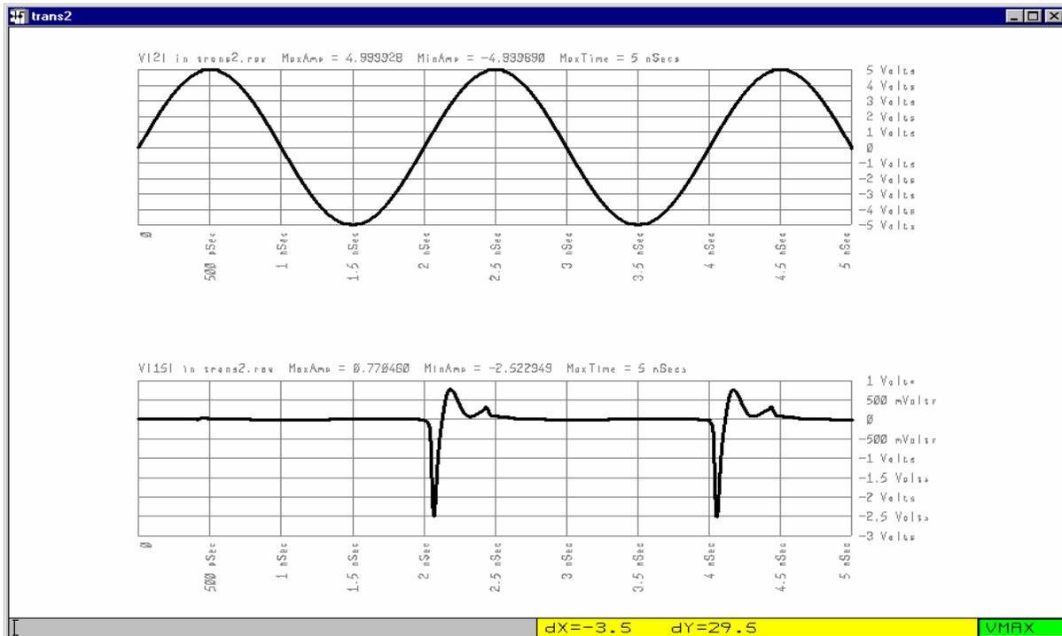
The predicted waveforms shown in the screen image above are taken from a circuit containing a step recovery diode. The input 500 MHz, 5 volts peak sine wave is applied across the silicon step recovery diode, and the characteristic sharp response is obtained at the output from the circuit.
