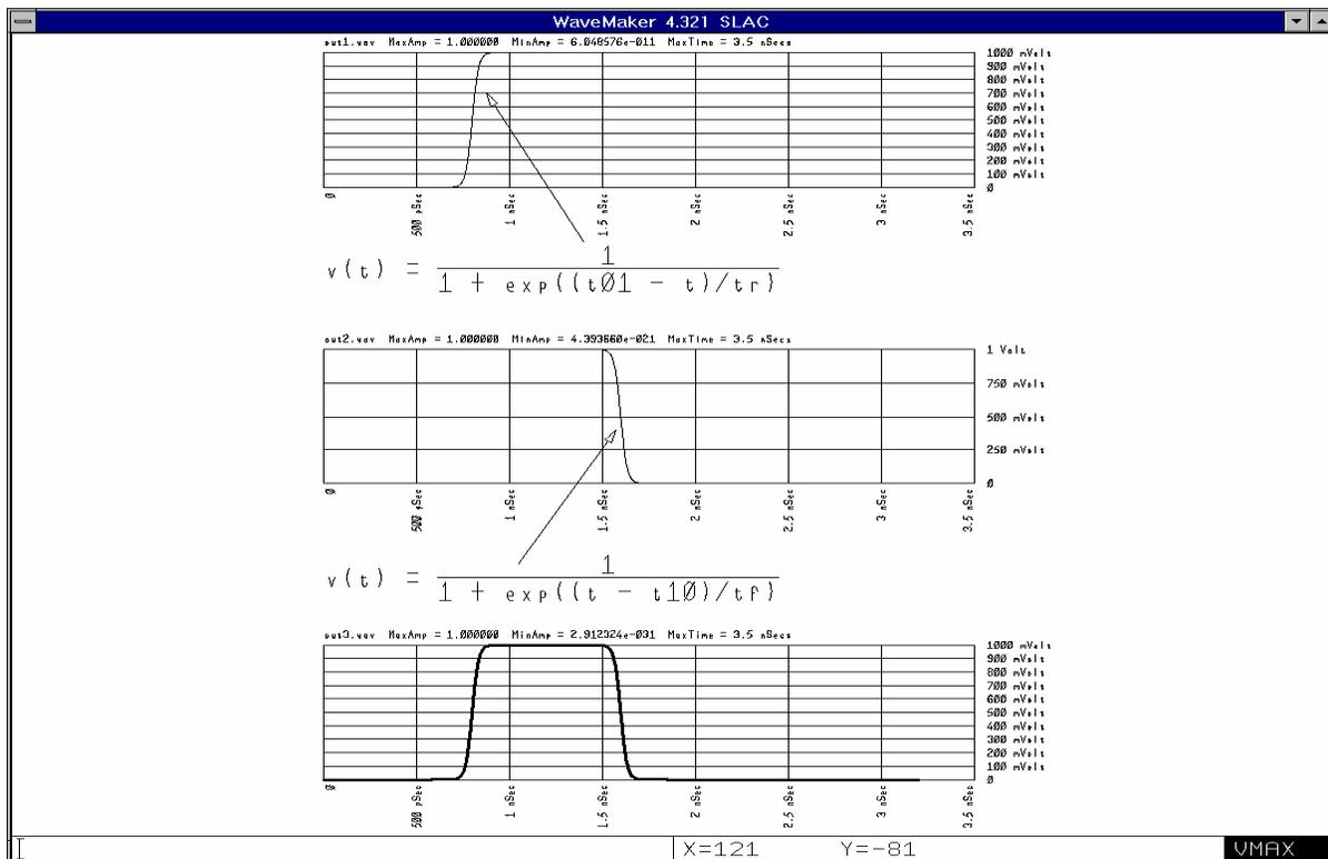
The schematic capture front end supports the generation of realistic waveforms, and the schematic definition of signal pre- and post-processing procedures.
