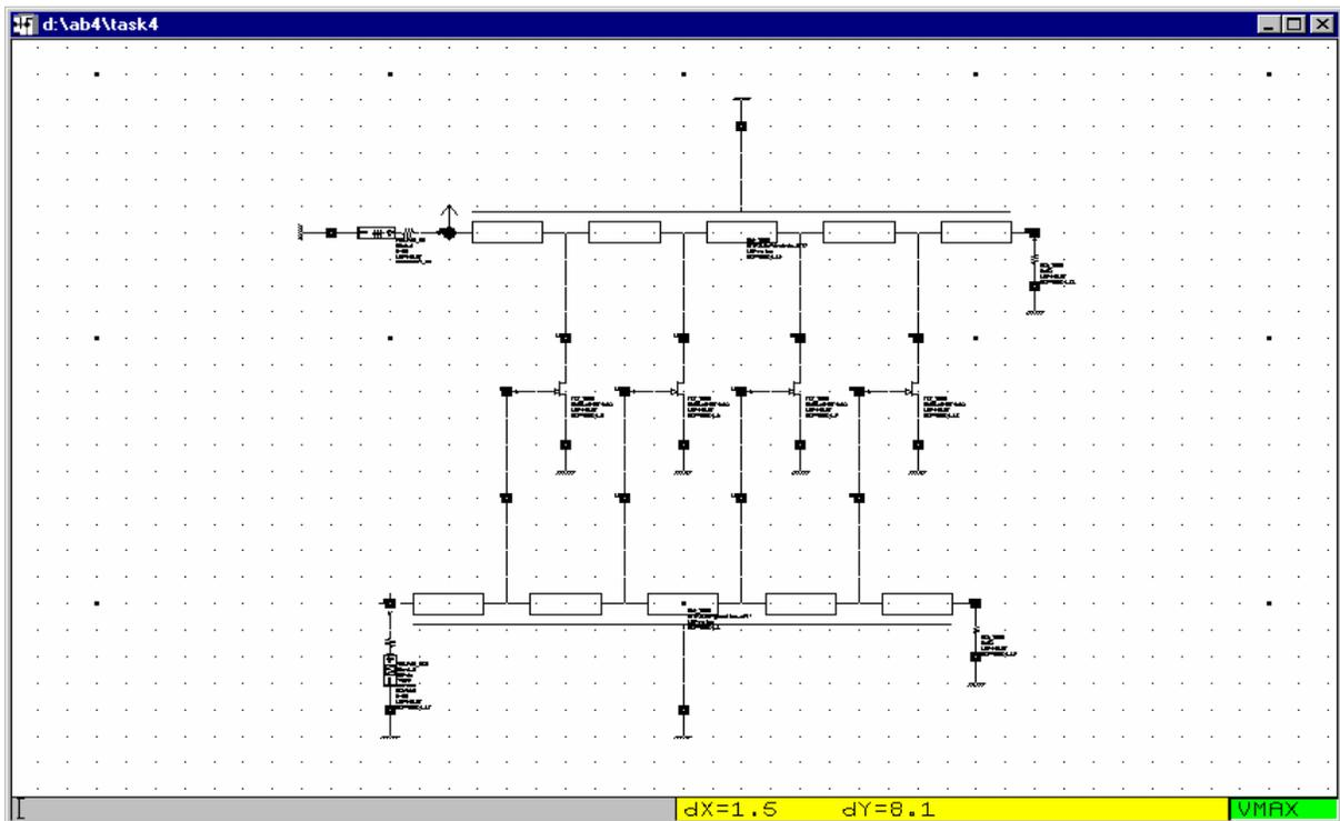
As an example, we will look at a very simple travelling wave amplifier circuit.
