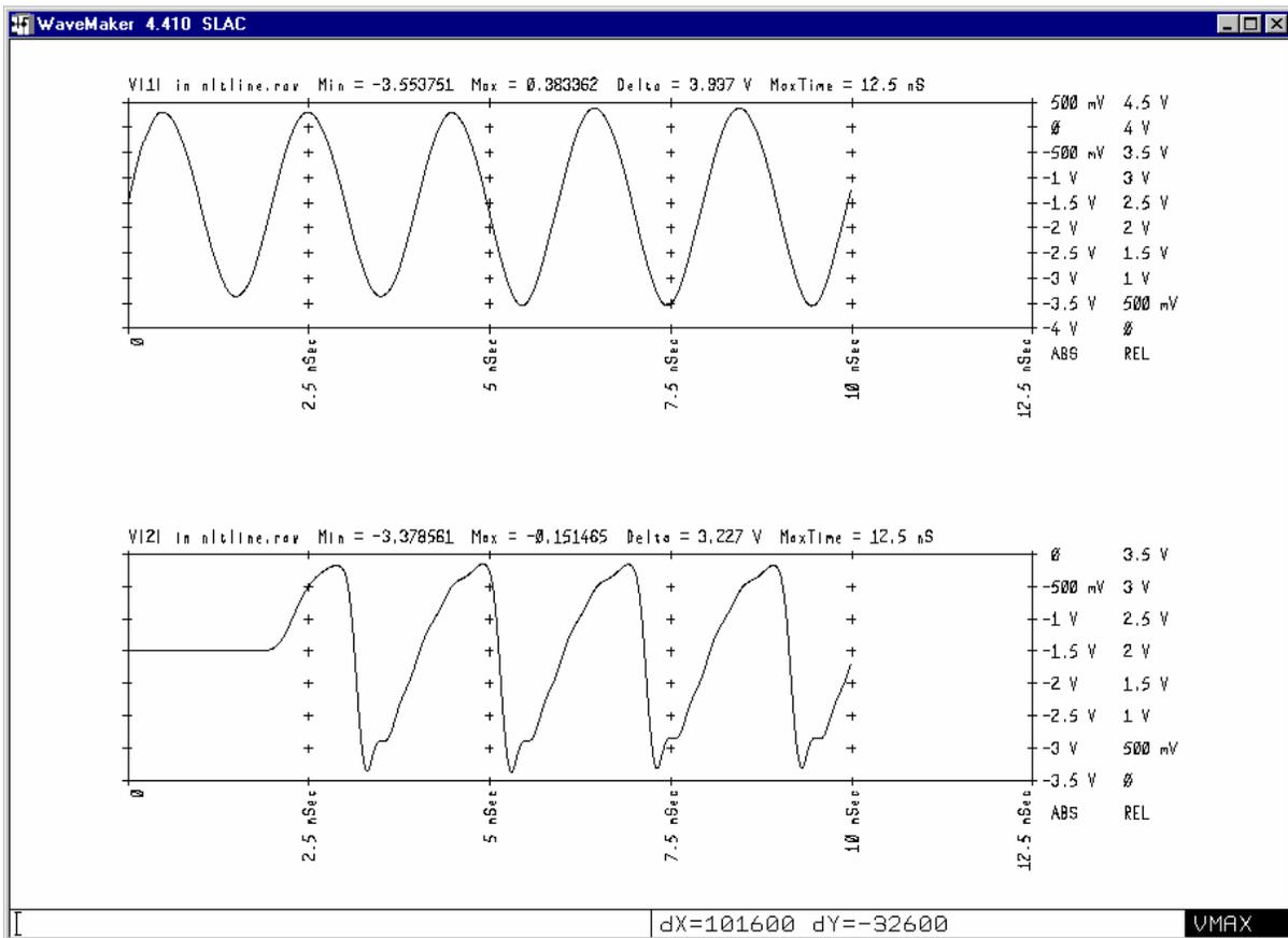
In the Non-Linear Transmission Line (NLTL), a series of Schottky barrier diodes (4 in schematic; 16 in the simulated response) are used to periodically load a coplanar transmission line. When a sine wave is sent down this line, the leading edge of the sine wave sharpens up, while the trailing edge displays a longer “fall time”. Again, many harmonics are associated with this non-linear phenomenon. The most important limiting factor is the skin effect losses of the passive transmission media.
