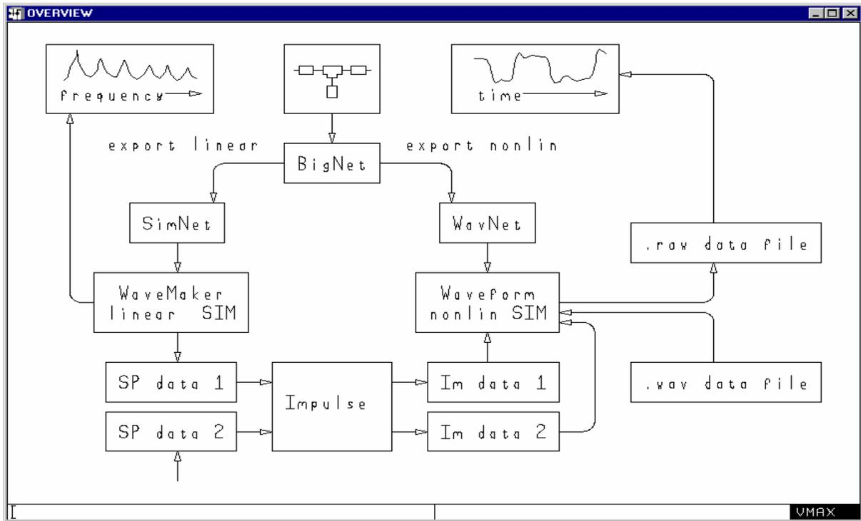
The linear and non-linear circuit netlist descriptions are derived from the same circuit schematic (the “BigNet” generalised netlist description).
