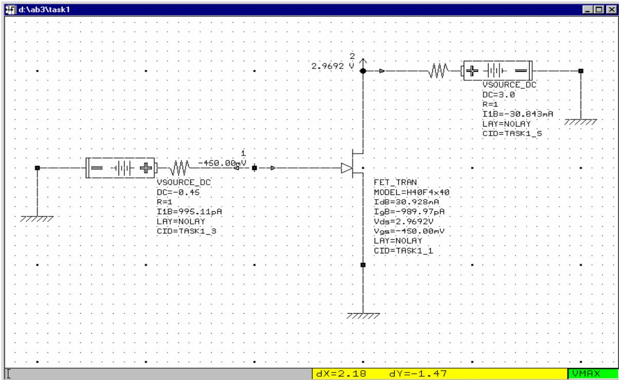
The bias voltages at each node in the circuit can be displayed on the circuit schematic, in addition to the quiescent current into each element, as shown above.
