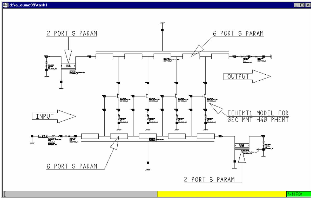
Use of S parameter data in GaAs travelling wave amplifier MMIC. The S parameter data is created through the use of an electromagnetics based simulator.
