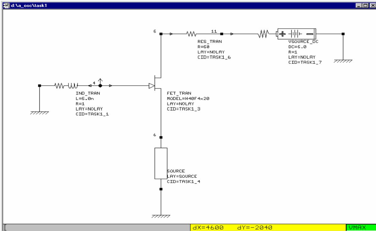
The circuit has an S parameter data section in the source of the GaAs PHEMT, and makes no use of injected pulses to start any possible circuit oscillations.
