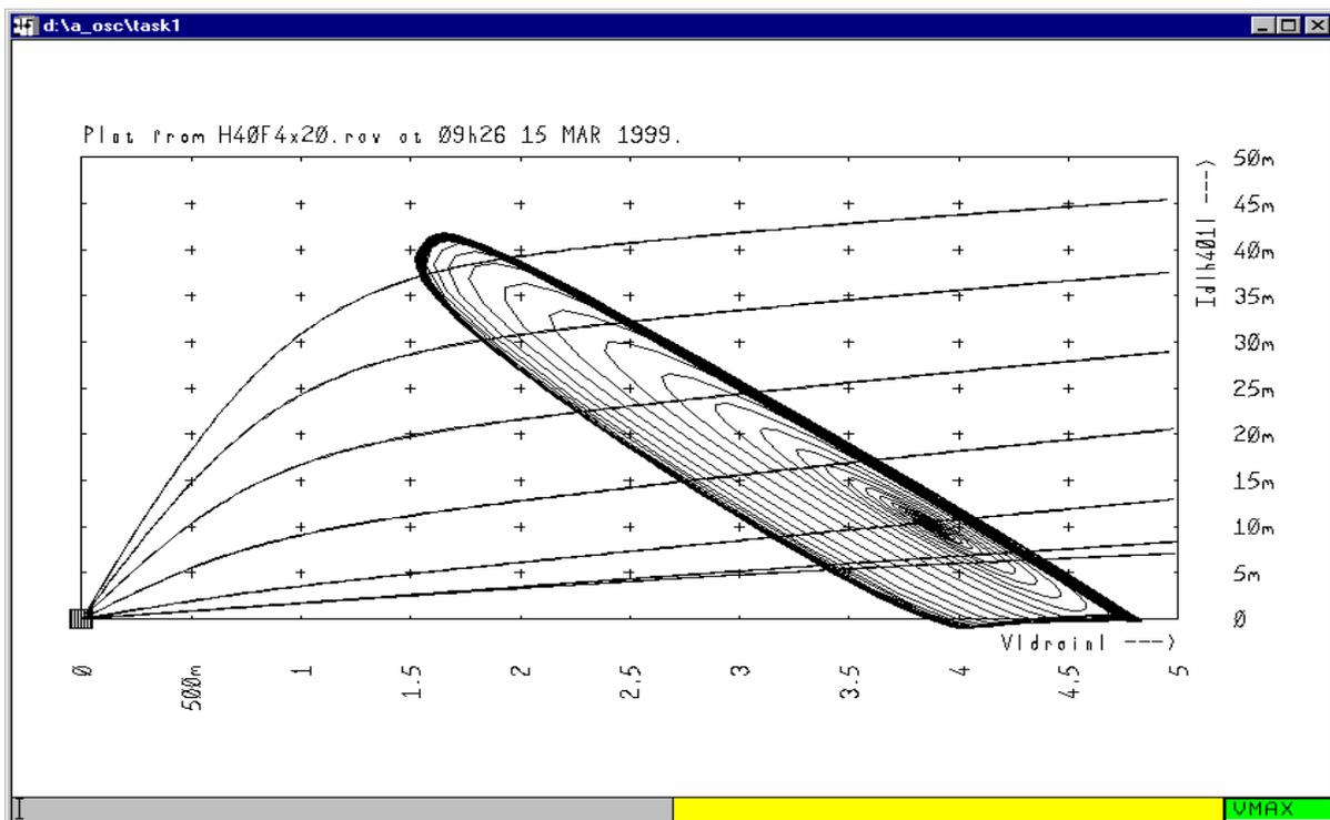
A fortunate consequence of the technique we use, which is different from that used in SPICE based simulators, is that there is always a low level random voltage signal at each node, very much analogous to the thermal noise present in any real electronic circuit. This low level signal, one microvolt or less in amplitude, causes the circuit to oscillate in situations in which it would unintentionally oscillate.
