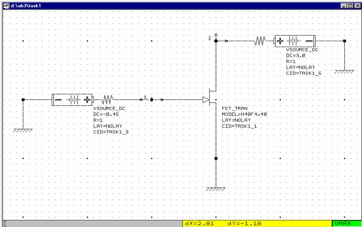
The non-linear circuit description requires the definition of all the biasing and signal source elements.
