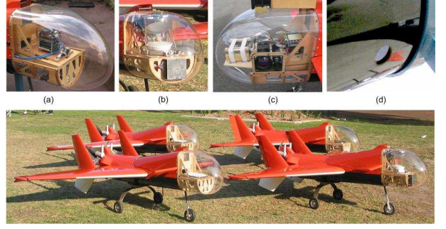
Figure 3: The replaceable nose cone of the Brumby Mk III UAVs is used to attach either an (a) SIS or (b) MMW radar or (c) colour and IR camera, or (d) a monochrome vision camera is fixed to the fuselage in down looking configuration.
