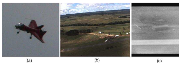
Figure 9: (a) The Brumby Mk III UAV in flight. It is equipped with a colour and an IR vision sensor. A (b) colour and (c) IR image frames showing different sections of the runway.
