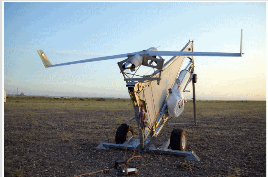
InSitu Scan Eagle Unmanned Aircraft on launcher, from uav_roadmap2005.pdf .
