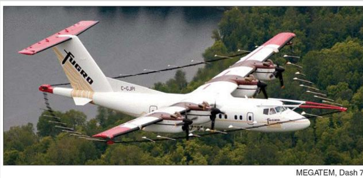
Fugro Airborne Services AEM aircraft fitted out with a large electromagnetic coil.
