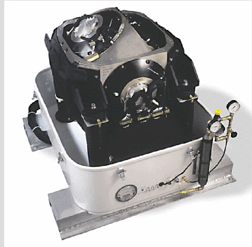
Gravity gradiometer: 350 kg+
