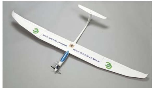
*The 8 foot wingspan CropCam Unmanned Air Vehicle used to photograph agricultural and forest lands. Images kindly supplied by [www.cropcam.com](http://www.cropcam.com) .*
