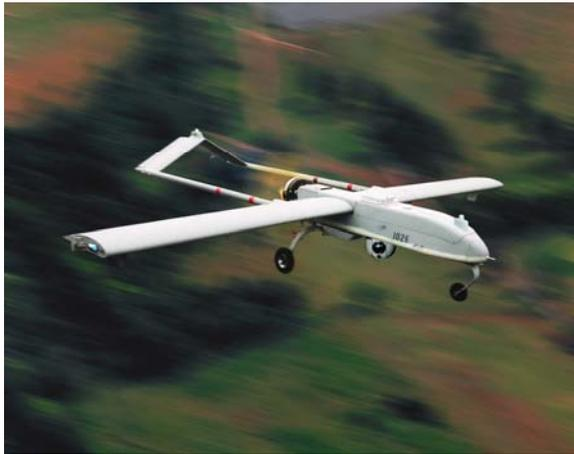
The AAI Shadow 200 UAV with a payload of 27 Kg, a take-off weight of 170 Kg and an estimated range of 600 Km. Image kindly supplied by [www.aaicorp.com](http://www.aaicorp.com).
