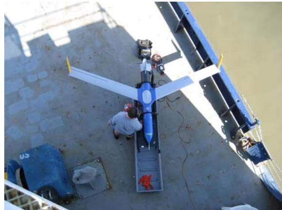
*The InSitu / Fugro GeoRanger UAV on a ship. The GeoRanger currently has a fuel and payload capacity of 5.4 Kg, a value that might change with ongoing developmental work. Image kindly supplied by [www.insitu.com](http://www.insitu.com) and [www.fugroairborne.com](http://www.fugroairborne.com).*
